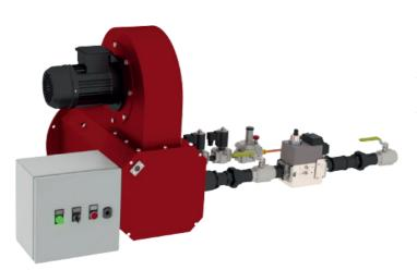
The 'TFR-HT' burner series of packaged gas burners have been specifically designed for the firing of high-temperature ovens. They are intended for application where the high process temperature prohibits the use of standard PC burners or where high-velocity tempering air is required. The TFR-HT burners are suitable for oven temperatures up to 900°C.
