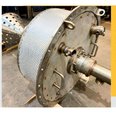
The 'FC' burner series of 'FUME CONE' gas burners have been specifically developed for fume incineration applications on a wide range of industrial plants; typical applications include the incineration of exhaust fumes from paint solvent and removal of smoke from curing ovens.
