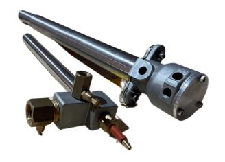
The GTS Comtherm pilot PB-FD series is equipped with a separate air and gas inlet. The mixing of the gas and air occurs inside the body of the burner, without the need of an separate air/gas mixer.
